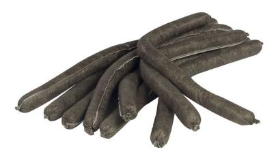
Universal absorbents will soak up just about any liquid spilled, including water. These "large" socks are sold 20 to a case, measure 3" in diameter and 8' in length, and are used to surround a spill to prevent it from spreading and causing further damage.
